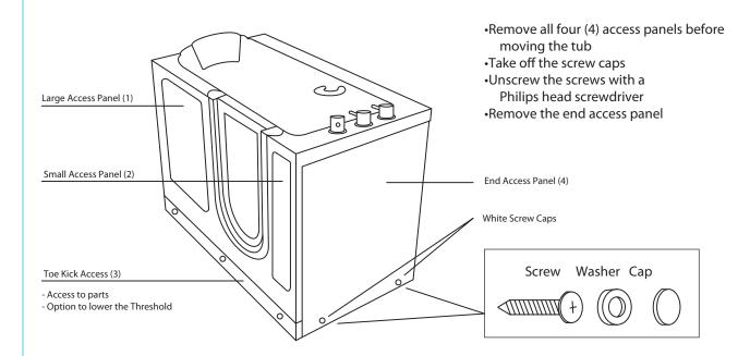
WARNING: Do not carry the walk in tub by the panels. Be careful when carrying the tub, avoid front panel contact with the floor or stairs to prevent damages. Make sure no loose parts are hanging down. Remove all four (4) access panels before carrying the tub to prevent them from falling out and breaking.
