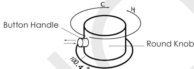
*\*The button knob stops here at 100.4 Fahrenheit. To adjust to a hotter temperature past 100.4 F, press the button knob in while turning the handle counter clockwise*
