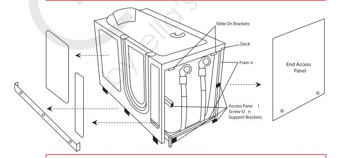
WARNING: Lift and carry the tub only by the frame. Protect the bottom of the tub to avoid breaking the shell.
