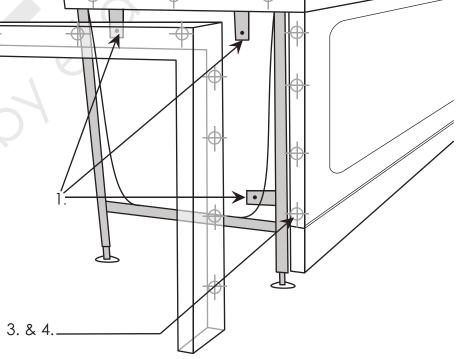
The extension kit can be installed as needed. Opening can be filled as desired.
